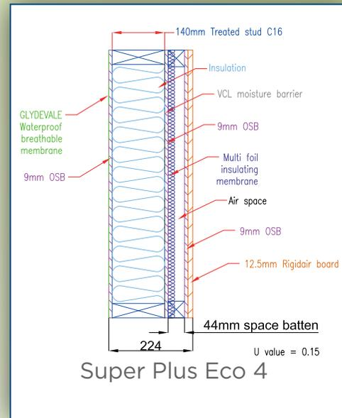
Shown here are section drawings of the six standard panels in the Eco Homes range together with a cut-through section of a Super Eco Plus 4 panel. Inside surfaces are faced with 12.5mm Rigidair board. This material is four times stronger than conventional gypsum board and is made from recycled paper. With high pull-out resistance and a ultra-smooth surface it does not require plastering and is ready to receive all forms of decoration with minimal preparation.
