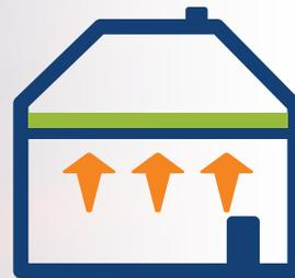
Warm air is buoyant, and warm air will rise, meaning extra insulation should be placed at the ceiling or roof.
