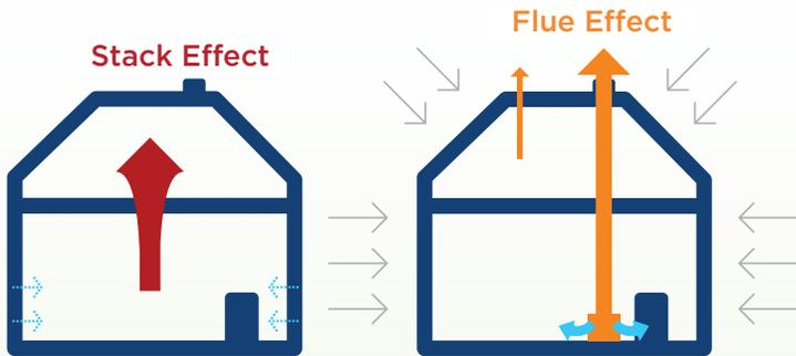
Air moves inside your house by the **stack effect**. This is the movement of warm air upwards, being replaced by cool air at the bottom of the house. This cool air could be drawn into the house through cracks and holes, gaps in floorboards or poorly fitting seals around windows and doors.
