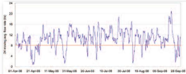
Graph of 24hr average stack flow from iPSV bathroom - with airtight buildings
